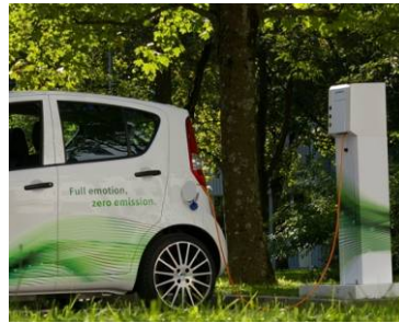
AC Charging Point
